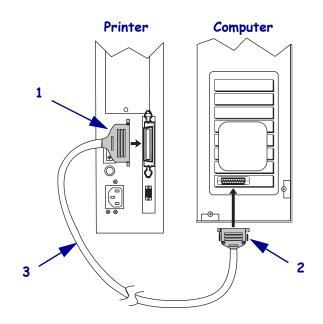
Figure 7 • Connecting the Printer through the Parallel Port
